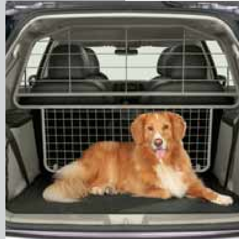
Separation rack Beige colour, behind 2nd row. Can be combined with trunk trays (MZ313027 and MZ313518). No curtain airbag interference. Removable by fly-nuts. With "ski-door" for long luggage MZ313098
