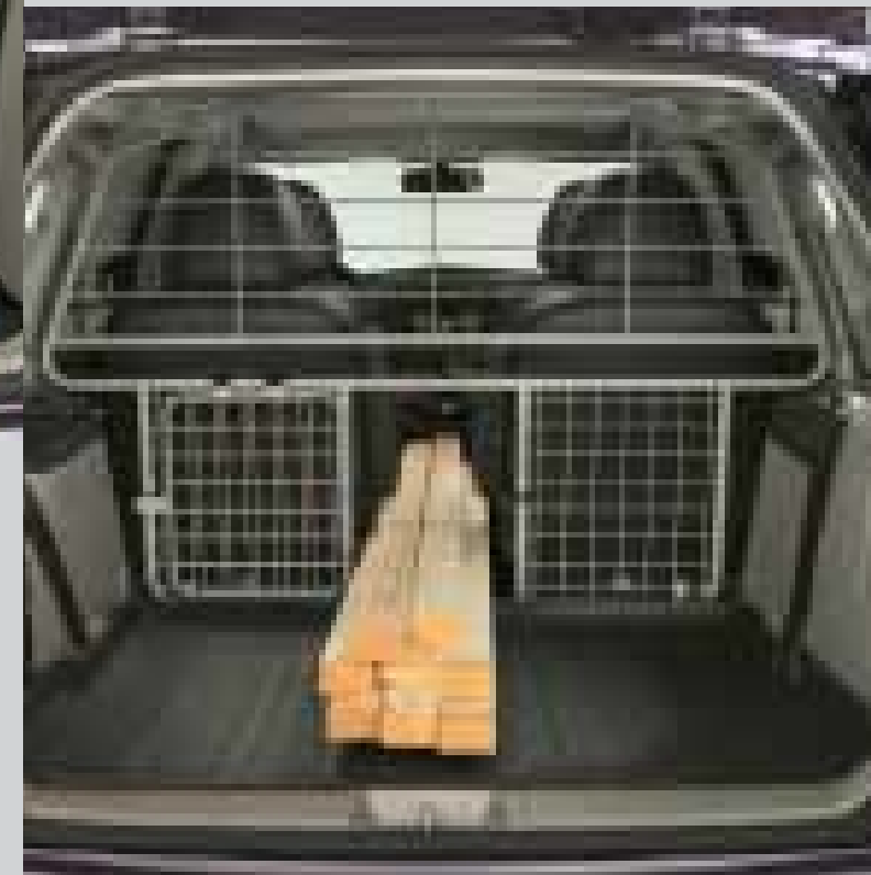
Separation rack Beige colour, behind 2nd row. Can be combined with trunk trays (MZ313027 and MZ313518). No curtain airbag interference. Removable by fly-nuts. With "ski-door" for long luggage MZ313098
